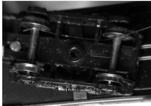
Insert the phosphor bronze wire as shown above. Two kinds of wires are supplied. The phosphor bronze wire is not coiled and is like a spring. Bend a hook in the wire as shown to secure the wire.
