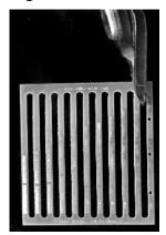
2. Free throw bar by cutting the the sprue parallel to the length of the tie.
